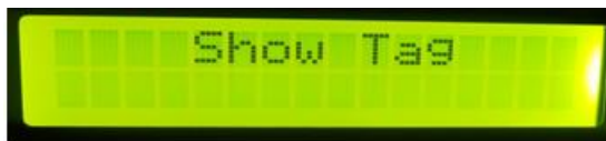
Fig.11. LCD display showing the message "Show Tag" once the user reaches the central lift for un parking a car
