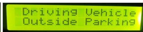
Fig.14. LCD displays the message before moving The parking slot to the central lift
