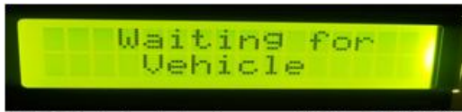
Fig.5. LCD display showing the message "Waiting for Vehicle" once the car reaches the central lift.
