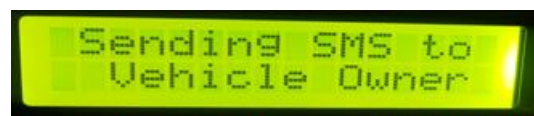
Fig.10. LCD display showing the message during the period when the car is moved from central lift to the slot.
