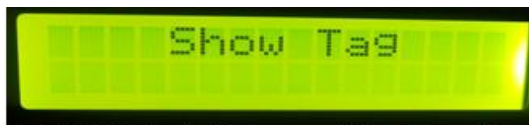
Fig.6. LCD display showing the message "Show Tag" once the car reaches the central lift once the system is initiated.
